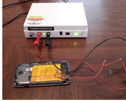
Fig. 1: Monsoon Mobile Device Power Monitor’s main channel measurement connection
