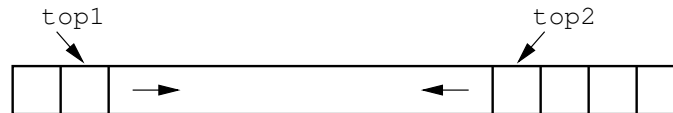
Figure 4.20 Two stacks implemented within in a single array, both growing toward the middle.
