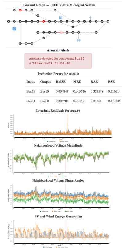
Fig. 8: illiad Dashboard - IEEE 33 Bus Microgrid
