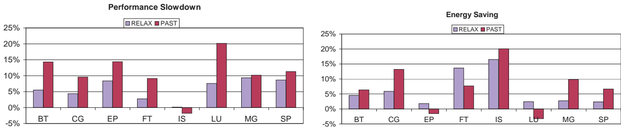
Figure 3. Performance slowdown and energy saving of CPU MISER when using the PAST algorithm and the RELAX algorithm with \lambda = 0.5 .
