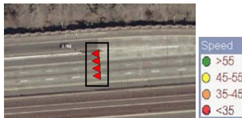
Figure 3. S_D map of detector speeds (MPH) at 10:50 AM on Feb 5, 2008. Black box shows traffic incident.
