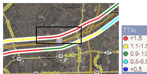
Figure 2. S_L map of I-66 link-level travel time index (TTAi) for Feb 5, 2008 at 10:50 AM. The black box shows the incident region.
