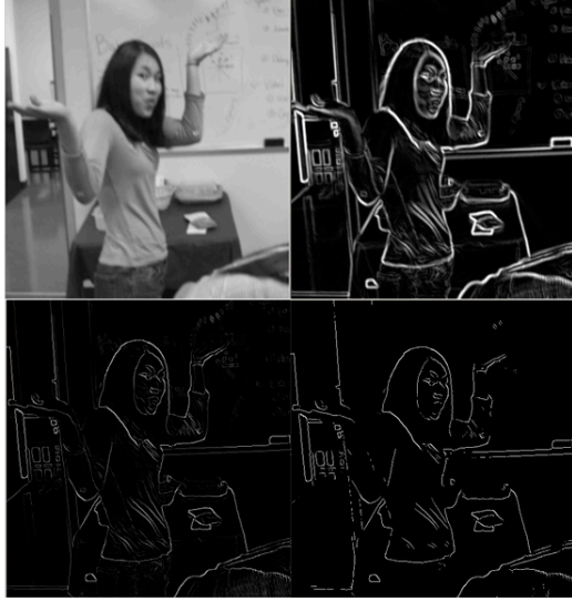
Figure 3. Four steps on Canny algorithm computation
